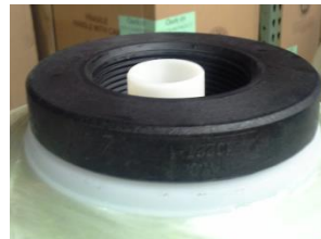
Figure 9: Centered Distributer Tube
