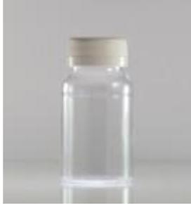
This 120mL bottle is specifically designed for the collection of water samples for **coliform bacteria**. This bottle includes sodium thiosulfate (either in a white pill form or powder) which deactivates chlorine up to 5ppm helping to ensure the survival of bacteria from sampling to testing. This bottle should only be filled to the 100mL line.
