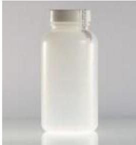
This 1,000mL sterilized bottle is used for the collection of lead and copper samples. **Lead and Copper** in water is usually caused by the corrosion of plumbing or equipment. Therefore, the best sample for detection is a “first draw” sample, or a sample taken immediately after the water has been sitting in the plumbing for at least six hours. Collecting 1,000mL of the “first draw” increases the chances of detecting Lead and Copper if it is from the plumbing.
