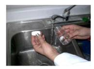
Remove the sealed cap from the sterile bottle. Please be careful not to touch the inside of the cap or bottle.
