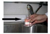
Fill the bottle up to the 100mL line on the sample bottle. Close cap securely without touching the inside of cap or bottle.
